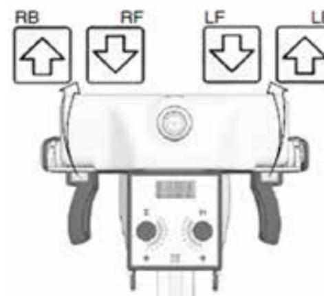
Easy controls to adjust the position of the unit when the Operator is in front of tube assembly.
