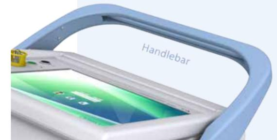
The handlebar internal sensors control the direction and speed of each wheel, proportional to the applied pressure.
